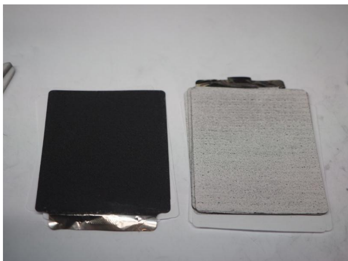
Figure 11: DUT ES26-42:1 after disassembly, the two distinct different sides of the electrode sheets
