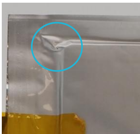
Figure 7: DUT ES26-42:2 before disassembly, close-up showing intentional hole in pouch
