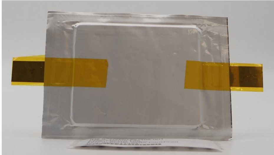
Figure 2: DUT ES26-42:1 before disassembly, back view
