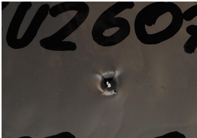
Figure 8: DUT ES26-42:2 before disassembly, close-up showing hole from nail penetration.
